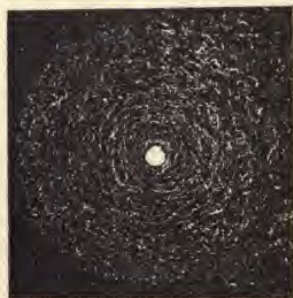
FIG. 325. — Iron Filings Arranged around a Conductor.
